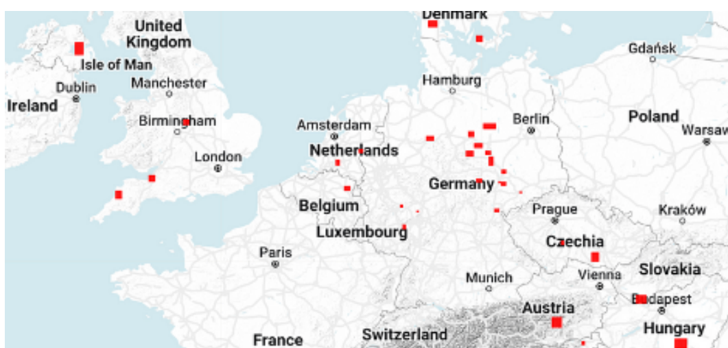
Figure 2. A sample of geometries covered in Kruitwagen et al.'s hand-labelled test set[? ]. Within each red geometry an exhaustive search for utility solar facilities was performed which produced a high quality and high confidence data set for testing purposes.
