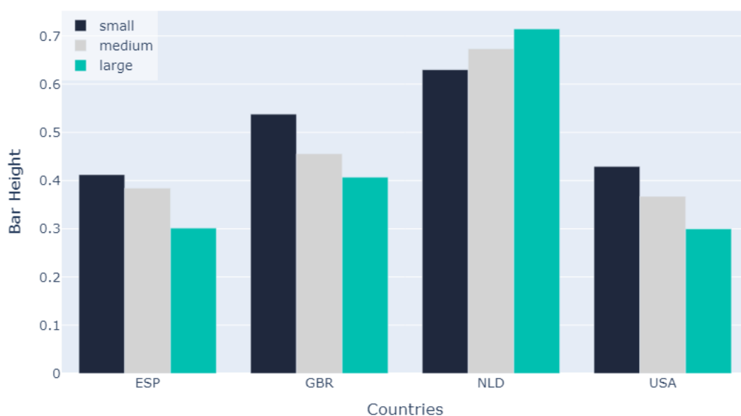
Figure 4. A comparison of four countries and their associated mean GCR for solar PV facilities of different sizes.
